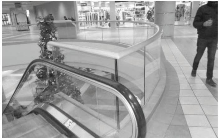
and step band must be adequately lit. According to A17.1/B44, floor-level illumination at the top and bottom landing areas must be at least 50 lux.
